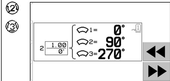
② ③ Apply Weights - Once the spindle is stopped, this screen shows the operator where to position the weights. During this phase, one weight should be placed at the zero position or all weights moved to the positions shown. Screens shown are for 3-weight balance, but the same process applies to 2-weight balance.
