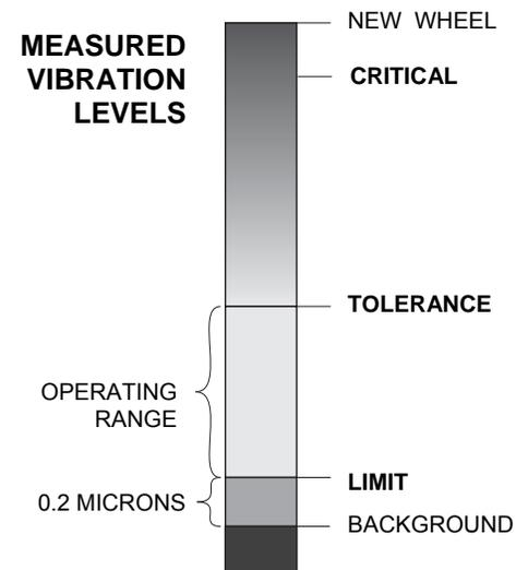
transmitted vibrations, these levels may change as adjacent machines are put into or out of service. **Set the balance Limit during periods when the system will receive the maximum floor transmitted vibration.**
