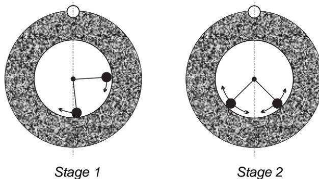
Stage 2: Find the correct angle for position of the masses in relation to the “center line”. Do this by moving the masses equally in different directions (one forward and one backward). Again, if the vibration level is increased, the opposite weight movement should be tried. This stage is complete when the vibration level can no longer be reduced.
