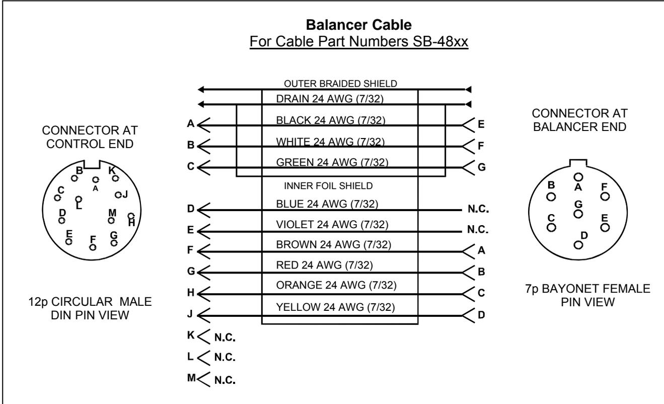
Sensor cable schematic
