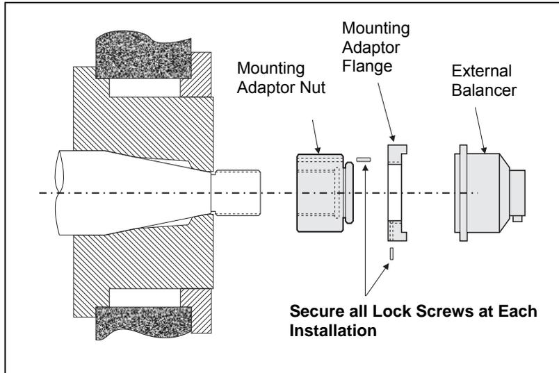
1. Loosen all lock screws before assembly. The engagement end of these screws should be below flush with the face of the adaptor/flange where they exit.
