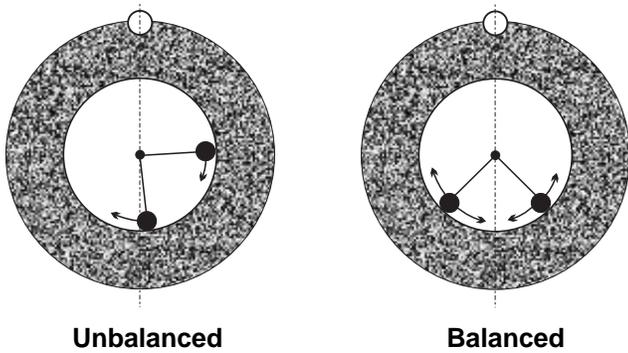
In order to correct for various and changing imbalances which occur on a user's grinding machine, the SBS Balance System uses two movable weighted masses, which can be independently positioned to compensate for any imbalance which is within the specifications of the system. These weights are located in the Balancer, and are driven by high torque electrical motors through a precision gear train.
