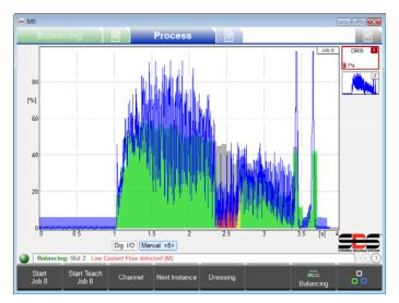
It is critical to understand that process screens always show the results of the most recently run current process. This means these screens will be blank when IVIS or the SB-5500 is started up, since there are no current process results to show.
