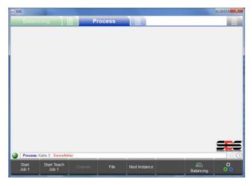
Successful connection of the IVIS program with the SB-5500 is indicated by the green dot (connection indicator) at the bottom left above the menu bar. Yellow color indicates connection is being attempted, and red color indicates a failed connection attempt. The Process and/or Balance View tabs for the installed products will also be displayed.
